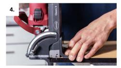
Align the machine and attach the stop square to the front edge for exact cutting.
