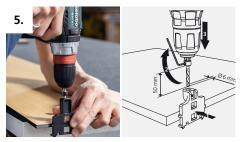
Using the drill and alignment jig, drill a 6 mm access hole into the surface.
