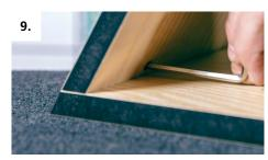
Tighten the Clamex S-20. Components can now be assembled and detached as often as required.
