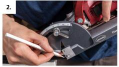
Carry over the position of the centre marking onto the first workpiece.
