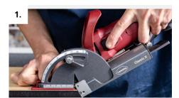
Cut 4 mm grooves into the edge.
