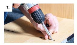
Fasten the connector halves with screws. For brittle materials, pre-drill 2 mm holes.
